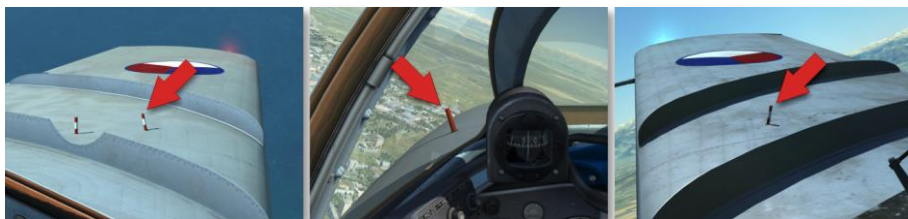
Figure 3.13. Mechanical indicators on the wings when landing gear is fully extended: left, nose, right
