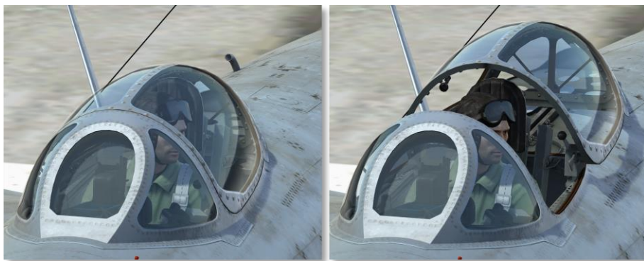
Figure 3.2. Closed (left) and opened (right) canopy
