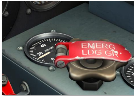
Figure 3.14. Pressure gauge and landing gear emergency extension valve handle on the right panel
